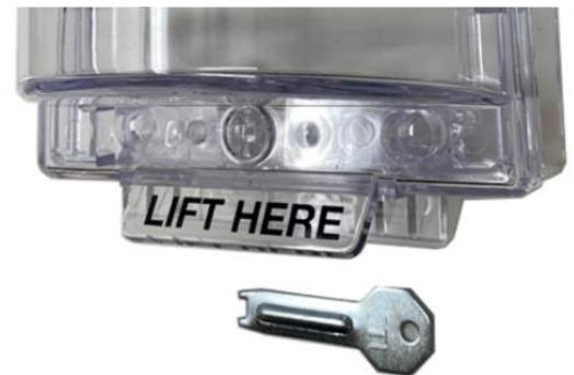
In an emergency, when considerable force is put on lifting the cover, the frangible lock in the front will break giving user access to button
