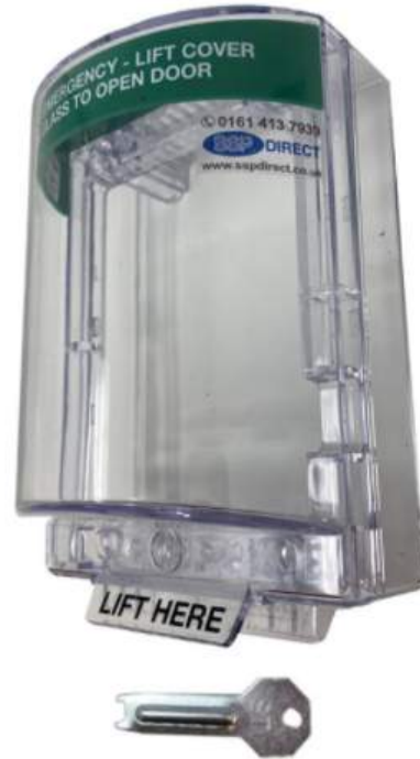
In an emergency, when considerable force is put on lifting the cover, the frangible lock in the front will break giving user access to button
